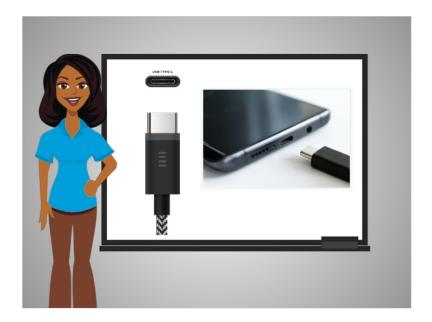
The USB-C port is like the USB port. It connects peripherals like mice and external storage to a computer, but it can also charge mobile and other tech devices.
